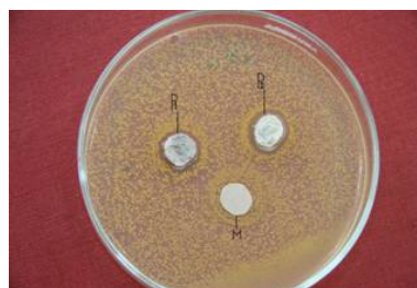
Fig. 2: Antibacterial test results using Staphylococcus aureus ATCC 25923 (P 1 -P b treated with AgNO 3 , P 2 -P a treated with AgNO 3 ).
