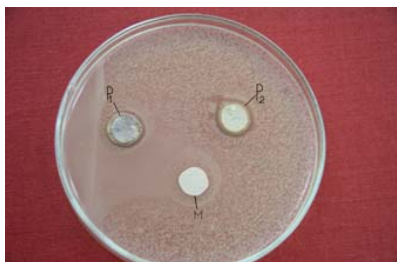
Fig. 1: Antibacterial test results using Escherichia coli ATCC 25922 (P 1 -P b treated with AgNO 3 , P 2 -P a treated with AgNO 3 ).
